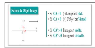
If  $\overline{SA} < 0$  the object is real If  $\overline{SA} > 0$ the object is virtual
