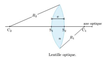
In the thin lens approximation, the vertices S1 and S2 are considered to coincide at a point O called the optical center. Two types of lenses are distinguished:
