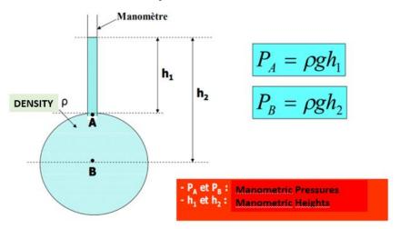
It is a device used only for measuring the pressures of liquids and not gases.
