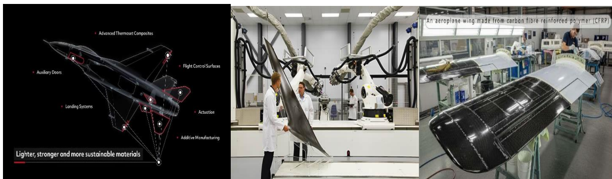
Figure 2.4 Advanced composite materials used in aerospace and high-performance engineering applications.
