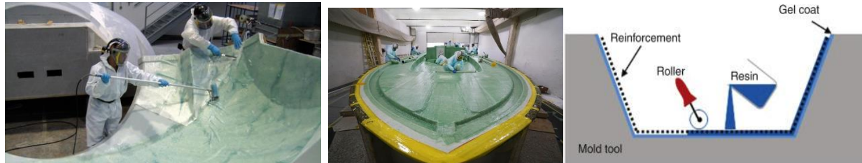
Figure 4.1 Schematic illustration of the hand lay-up process.
