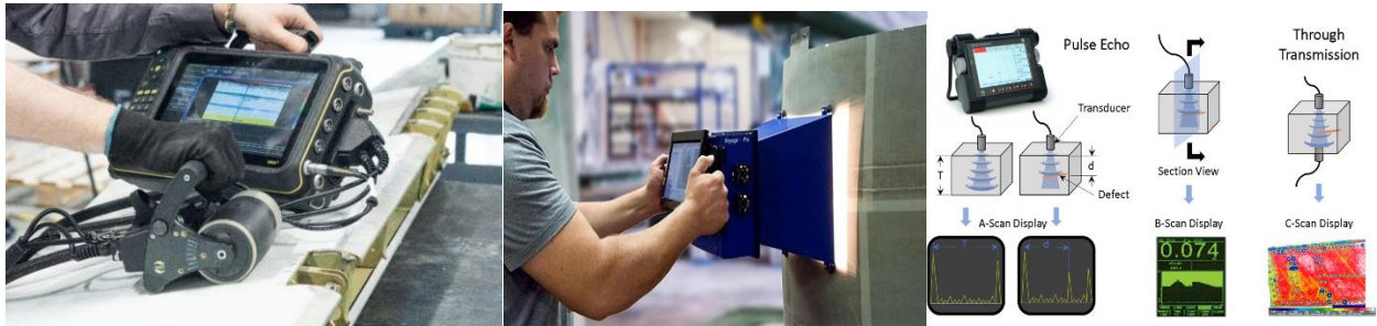
Figure 4.12 Non-destructive testing methods for composite inspection
