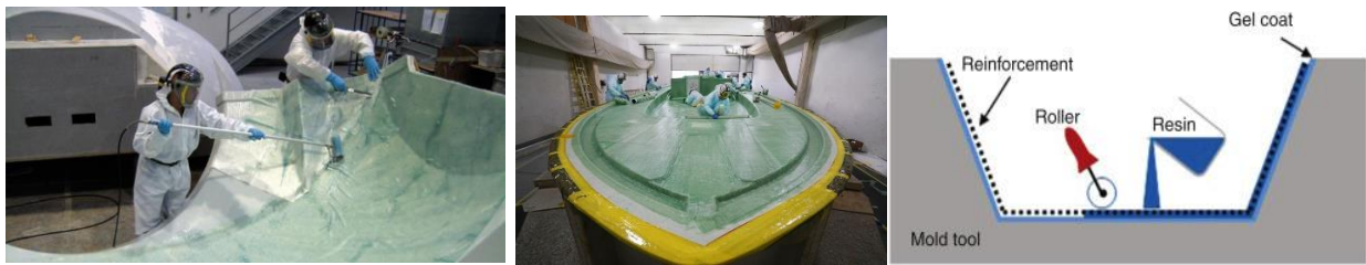
Figure 4.1 Schematic illustration of the hand lay-up process.
