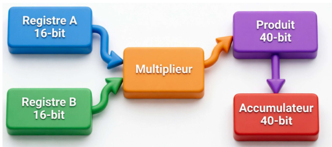
Figure 2.2 – Unité MAC : D = D + (A \times B)
