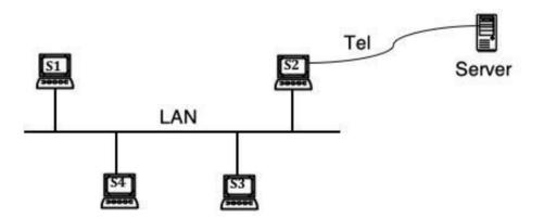
Stations S<sub>1</sub>, S<sub>2</sub>, S<sub>3</sub>, S<sub>4</sub> are linked by a local bus network offering a throughput of 10 Mbits/s. The station S2 is connected to an Internet access server by a phone link whose frequency band is [300-3400 Hz]. Given that the line rate is 62 Kbits/s:
