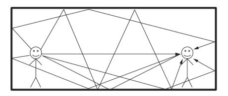
The absorption coefficient alpha is a measure of the sound absorption capacity of a material. It is defined as the ratio of the absorbed sound power to the incident sound power. Materials with high alpha values absorb more sound and reduce the level of noise
