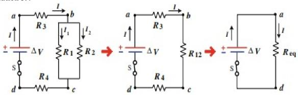
We can simplify the circuit by the rule of adding resistances in series and in parallel in steps. The resistors R<sub>1</sub> and R<sub>2</sub> are in parallel and their equivalent resistance R<sub>12</sub> between b and c is:
