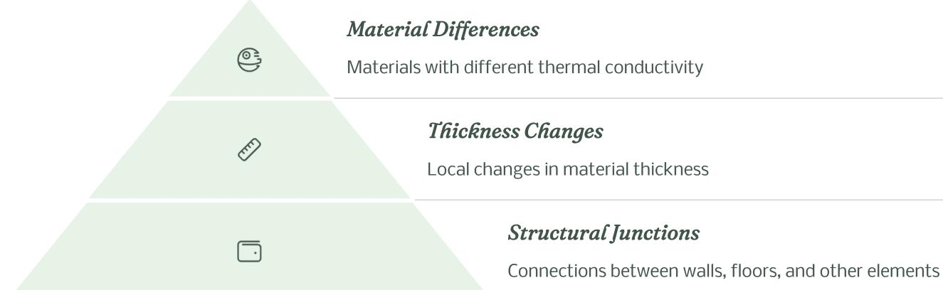
Thermal bridges occur where the insulation layer is discontinuous. According to Roulet (2016), avoiding thermal bridges is imperative but not always possible.
