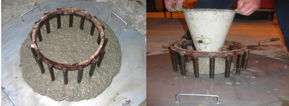
*Figure I.7 Essai J-Ring*
