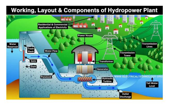
Water flows through dam → Water turns turbines → Turbines generate energy →
