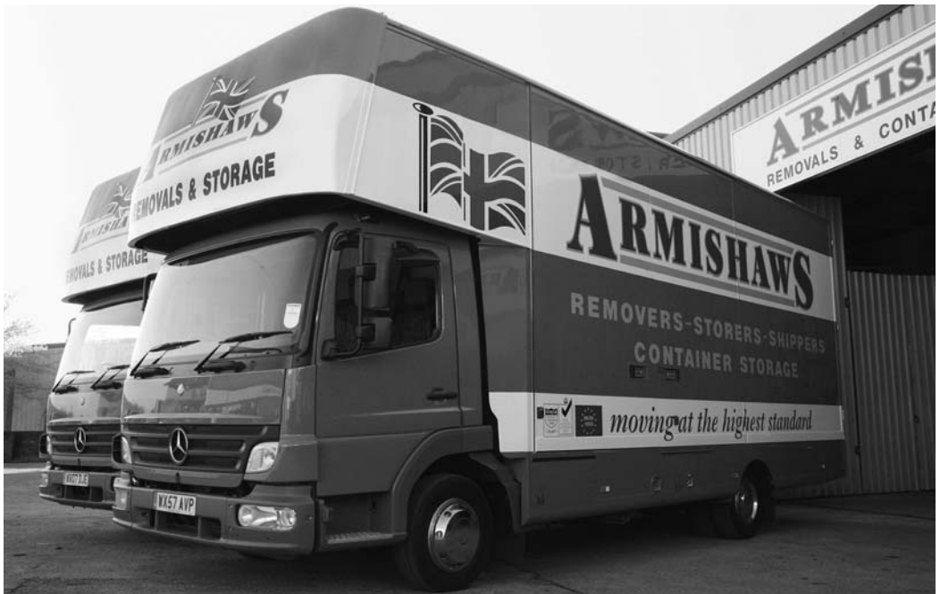
Figure 26.11 A rigid vehicle fitted with a high cubic capacity body for high volume/low weight cargo, which in this case are household goods (courtesy of Mercedes-Benz UK Ltd)
