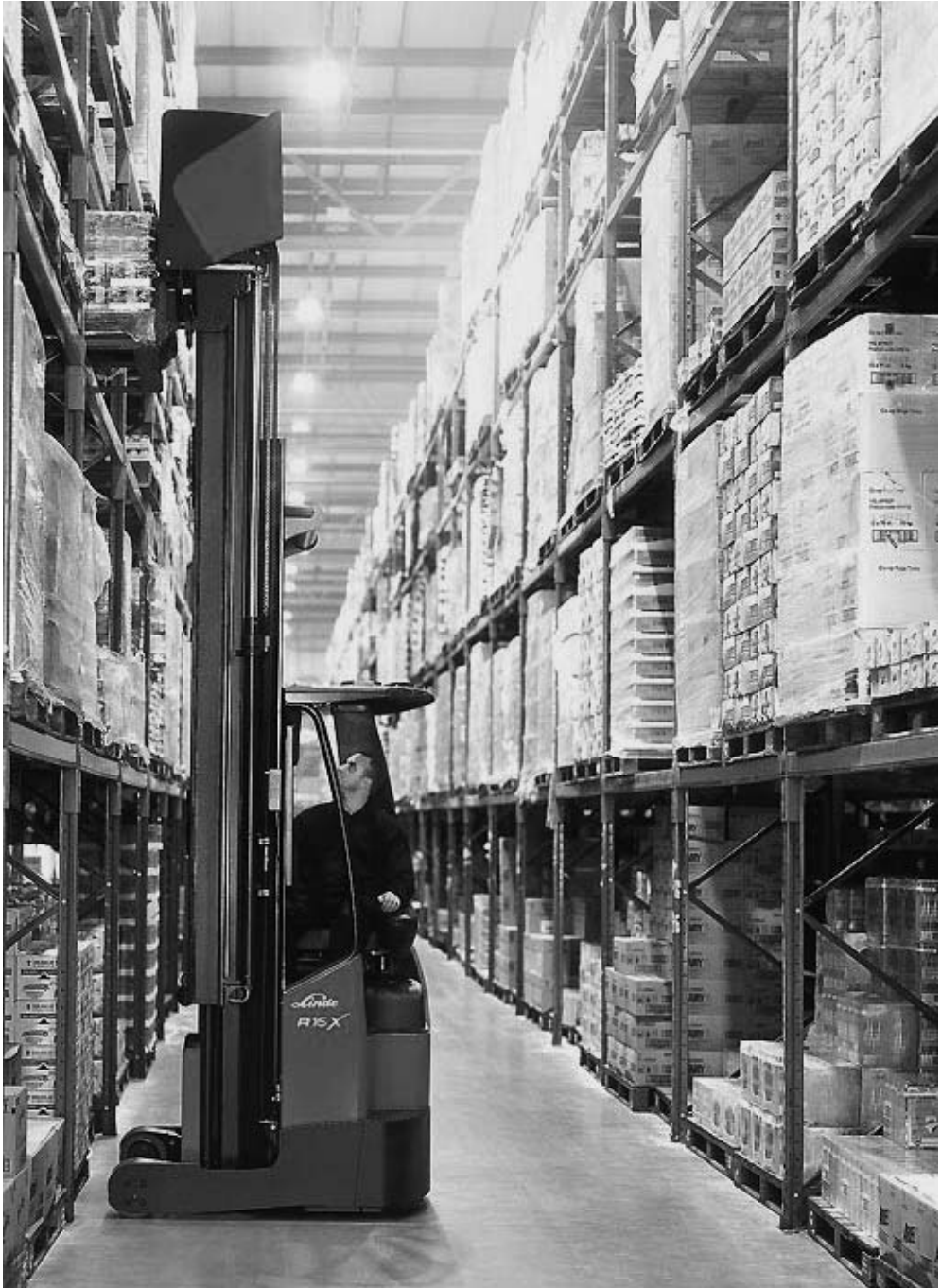
Figure 16.5 Adjustable pallet racking, being served by reach truck (courtesy of Linde)
