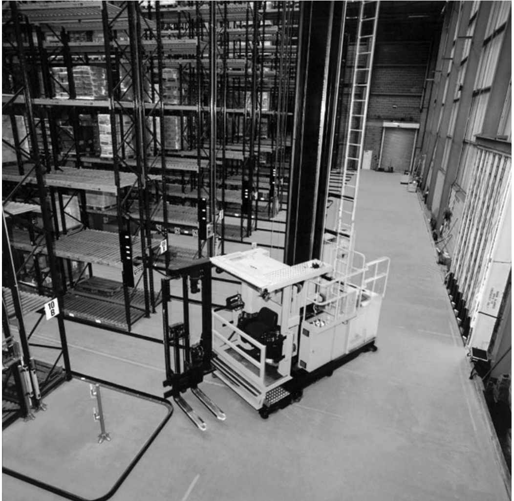
Figure 16.6 Narrow-aisle truck, with automatic aisle changing (courtesy of FKI Logistex)
