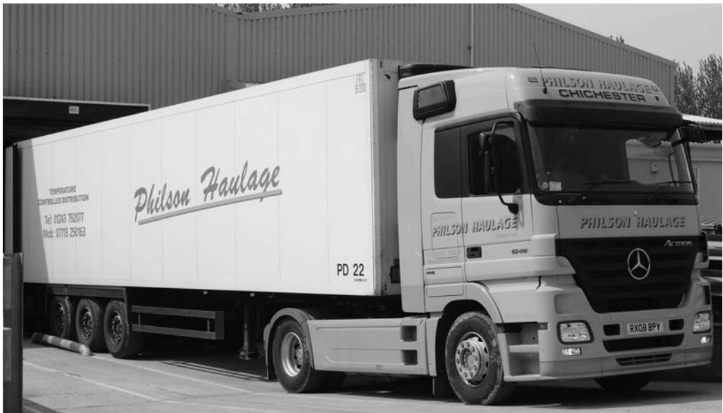
Figure 26.8 An articulated combination featuring a box trailer, which in this case is refrigerated (courtesy of Mercedes-Benz UK Ltd)
