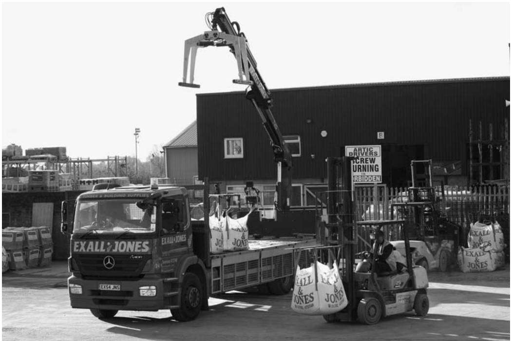
Figure 26.9 A platform or flat bed rigid vehicle with drop sides, which in this case is fitted with its own crane to assist loading and unloading (courtesy of Mercedes-Benz UK Ltd)
