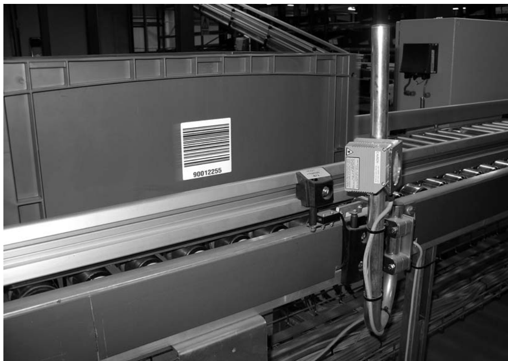
Figure 21.4 Automatic bar code scanning of plastic tote box (courtesy of Swisslog)
