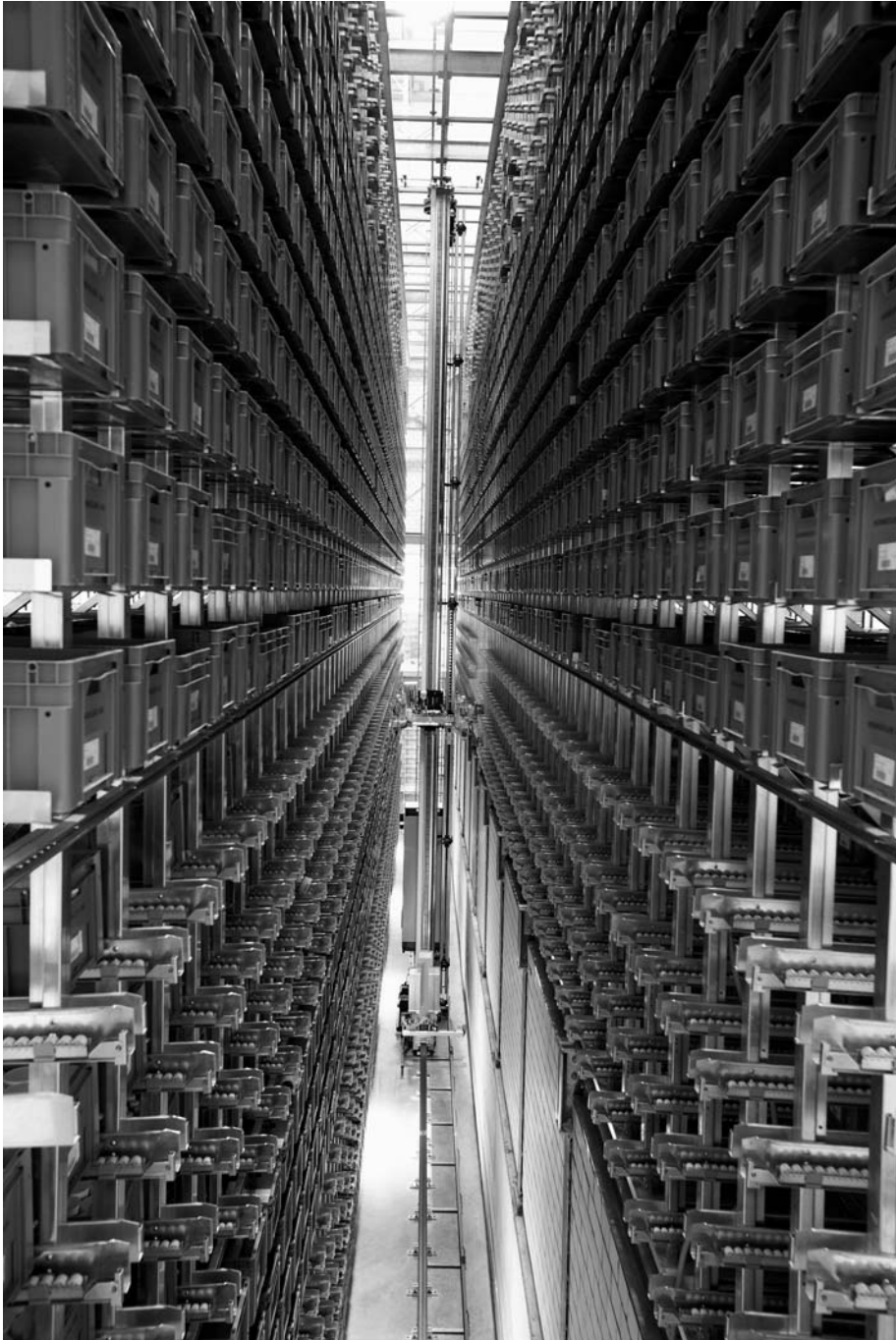
Figure 17.4 Miniload (courtesy of Jungheinrich)
