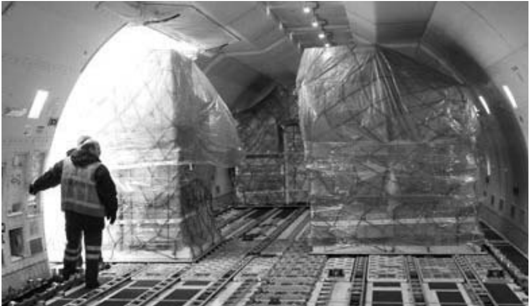
Figure 24.1 Air cargo pallets being loaded on to an air freighter (courtesy of Cargolux)
