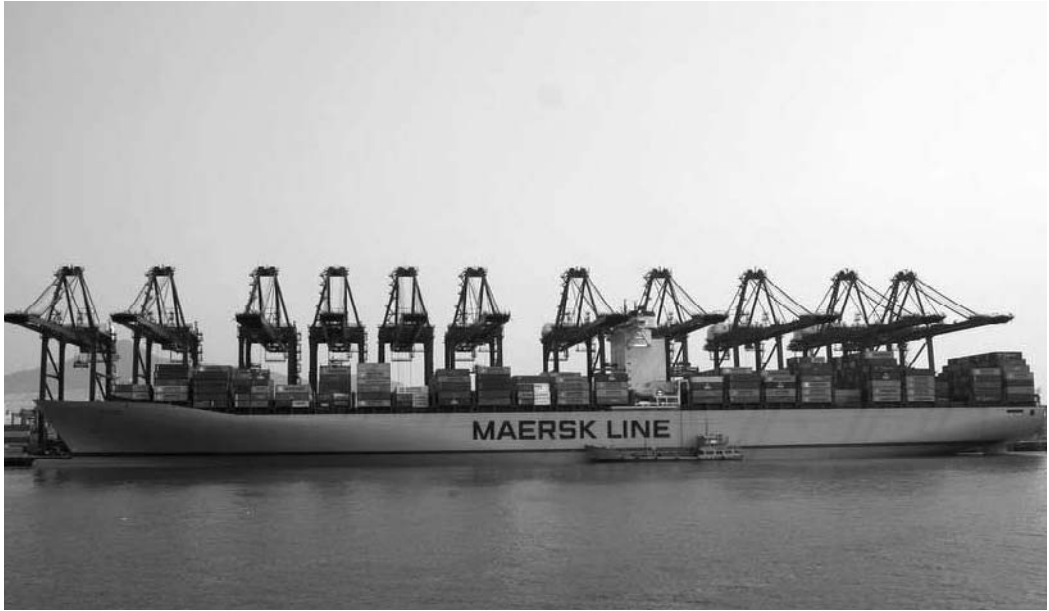
Figure 23.2 The Emma Maersk : the largest cellular container vessel in the world, capable of transporting 11,000 TEU
