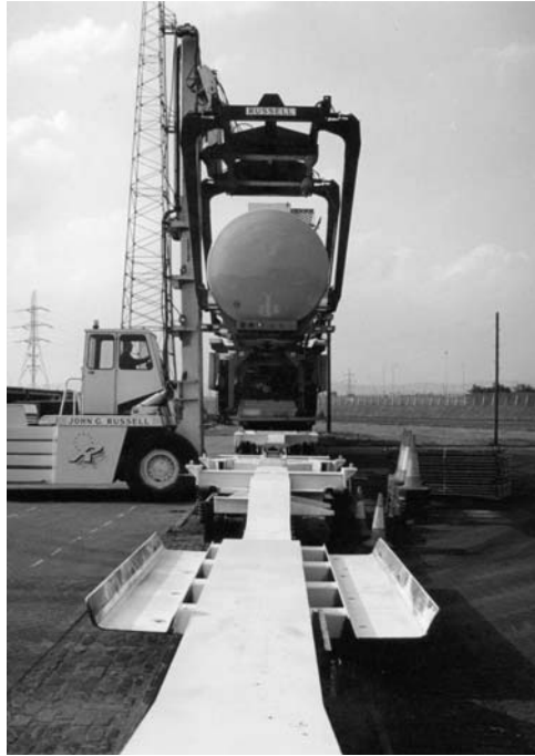
Figure 25.1 Spine wagons being loaded by a reach stacker equipped with a grapple (courtesy of John G Russell (Transport) Ltd)
