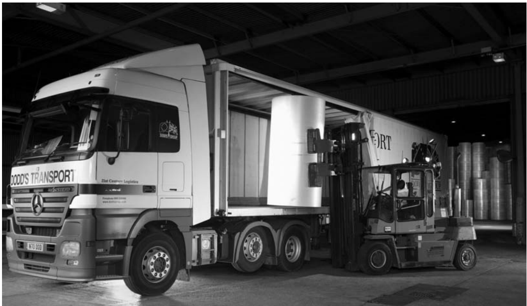
Figure 26.10 A curtain-sided trailer giving ease of access for loading (courtesy of Mercedes-Benz UK Ltd)
