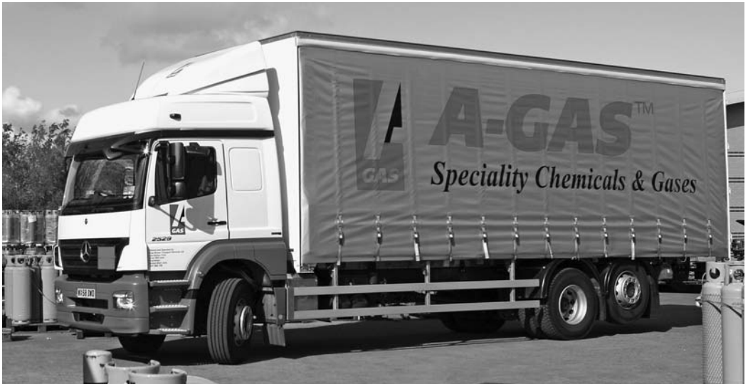
Figure 26.2 A six-wheeled rigid vehicle fitted with a lifting rear axle (courtesy of Mercedes-Benz UK Ltd)
