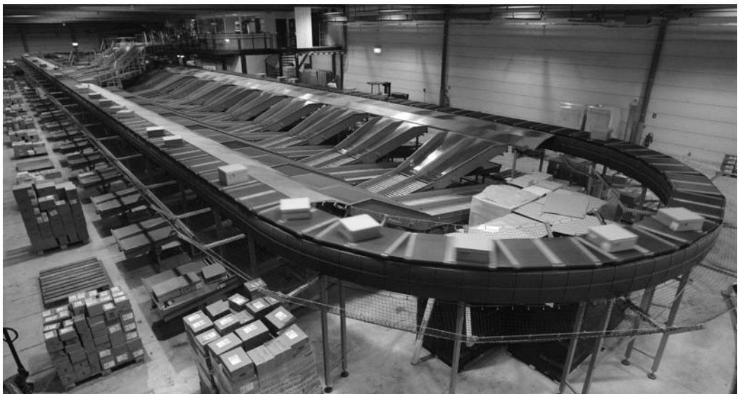
Figure 18.5 Cross-belt sorter (courtesy of Vanderlande)
