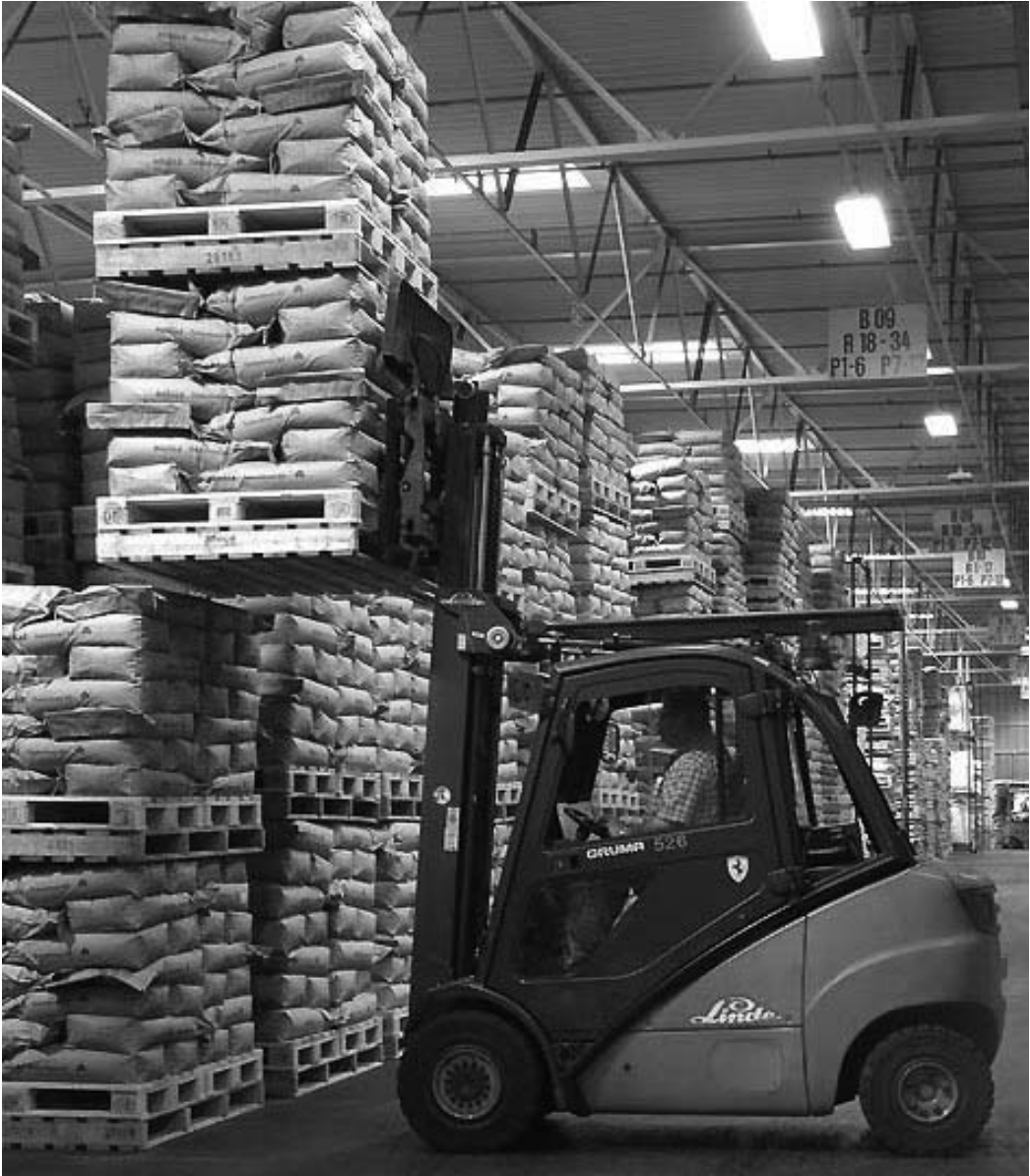
Figure 16.2 Counterbalanced fork-lift truck placing goods into a block stack (courtesy of Linde)
