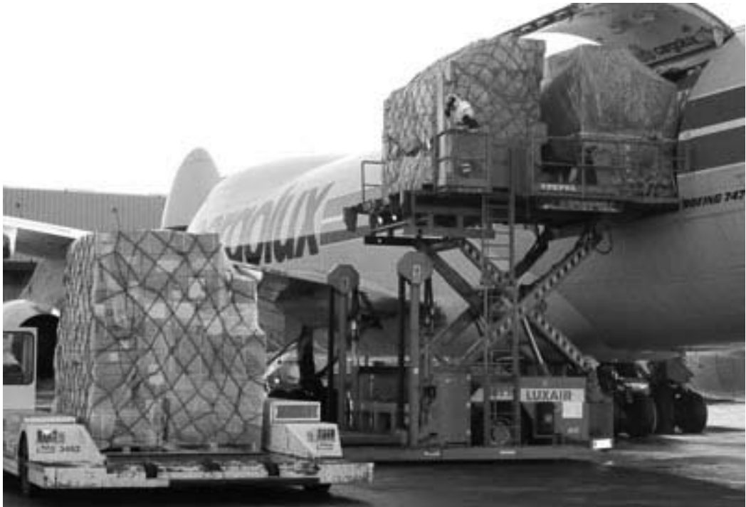
Figure 24.2 A Cargolux air freighter being loaded through the side door (courtesy of Cargolux)
