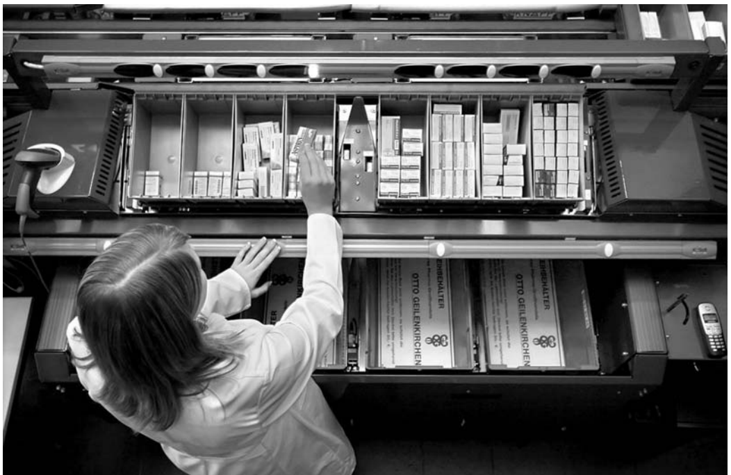
Figure 18.3 Totes-to-picker system (courtesy of Knapp)
