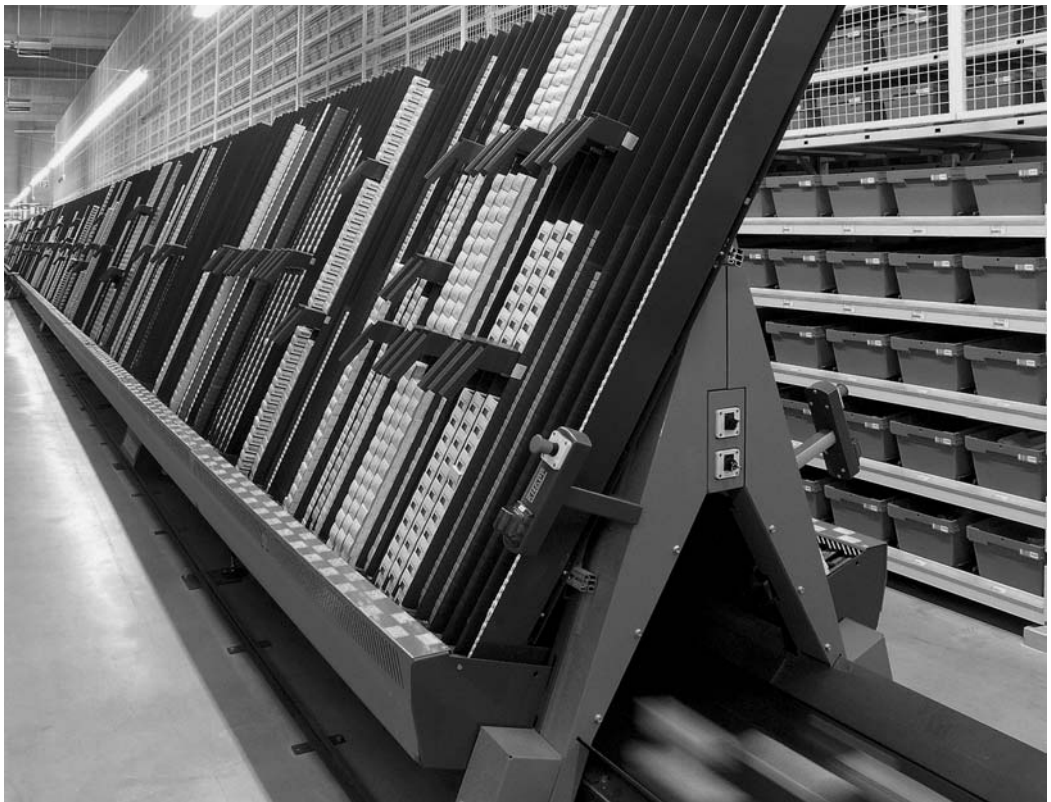
Figure 18.4 A-frame dispenser (courtesy of Knapp)
