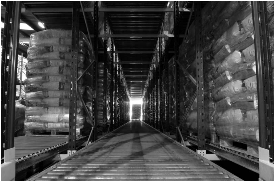
Figure 16.7 Pallet live storage (courtesy of Link 51)
