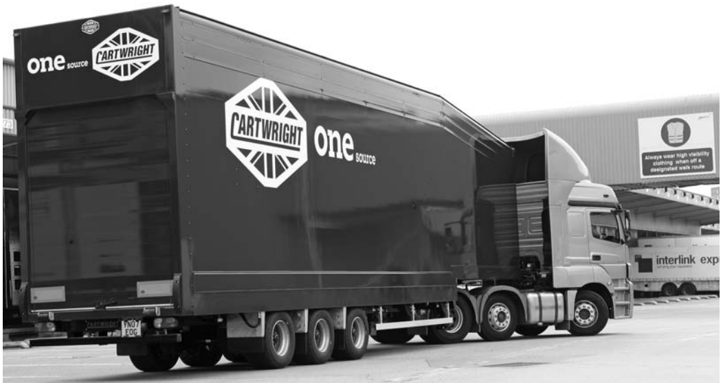
Figure 26.4 An articulated vehicle featuring a double-deck trailer (courtesy of Mercedes-Benz UK Ltd)
