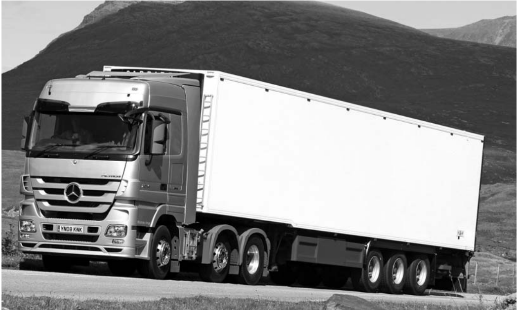
Figure 26.1 An articulated vehicle comprising a tractor and semi-trailer (courtesy of Mercedes-Benz UK Ltd)
