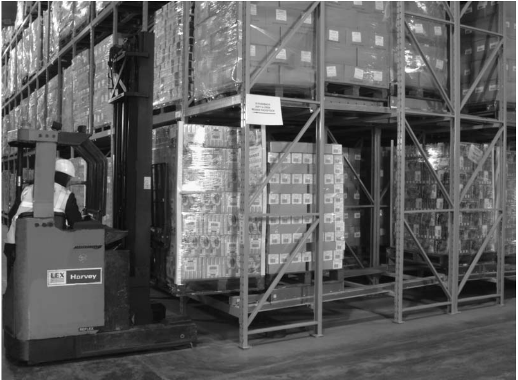
Figure 16.4 Push-back racking, being served by reach truck (courtesy of Redirack)
