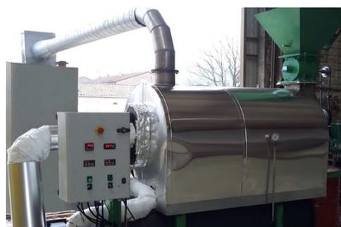
*The CarboChar-1, a pyrolysis machine for biochar production*
