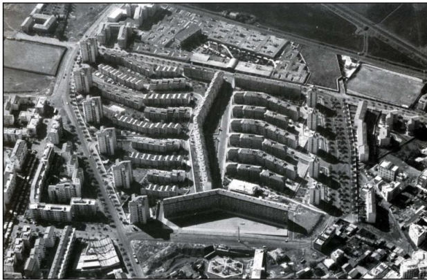
Figure 2. Aerial photograph of the Ina-Casa neighbourhood of Tuscolano, just after it was built. At the bottom is the church still under construction. Note the market square (bottom), the central spine of buildings in the shape of a 'boomerang' and the double system of encircling tower blocks.
