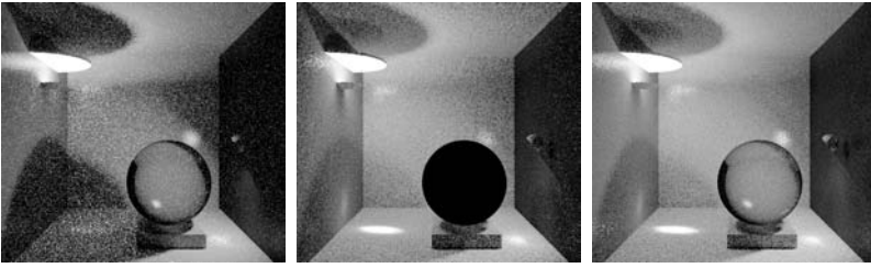
Figure 7.5. Left: stochastic ray tracing; middle: light tracing; right: bidirectional ray tracing. (Courtesy of F. Suykens-DeLaet, Dept. of Computer Science, K. U. Leuven.) (See Plate V.)
