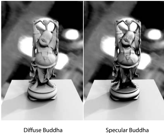
Figure 8.20. Diffuse and glossy Buddha rendered using PRT with separable BRDFs for high-frequency illumination. (Image courtesy Peter-Pike Sloan and John Snyder.) (See Plate XXV.)
