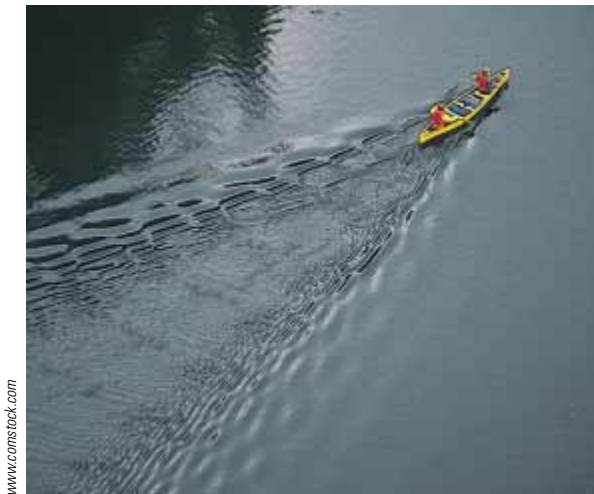
Figure 17.11 The V-shaped bow wave of a boat is formed because the boat speed is greater than the speed of the water waves it generates. A bow wave is analogous to a shock wave formed by an airplane traveling faster than sound.
