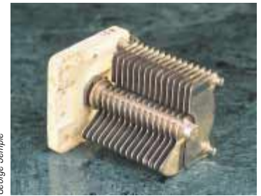
Figure 26.18 A variable capacitor. When one set of metal plates is rotated so as to lie between a fixed set of plates, the capacitance of the device changes.
