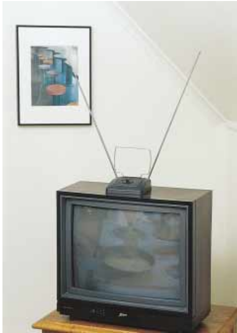
Figure Q34.12 Questions 12, 14, 15, and 16, and Problem 49. The V-shaped pair of long rods is the VHF antenna and the loop is the UHF antenna.
