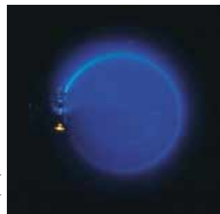
Figure 29.20 (Example 29.7) The bending of an electron beam in a magnetic field.
