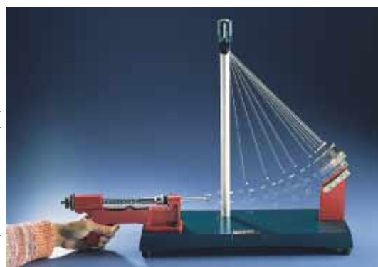
Figure 9.11 (Example 9.7) (a) Diagram of a ballistic pendulum. Note that v_{1A} is the velocity of the bullet just before the collision and v_B is the velocity of the bullet–block system just after the perfectly inelastic collision. (b) Multi-flash photograph of a ballistic pendulum used in the laboratory.
