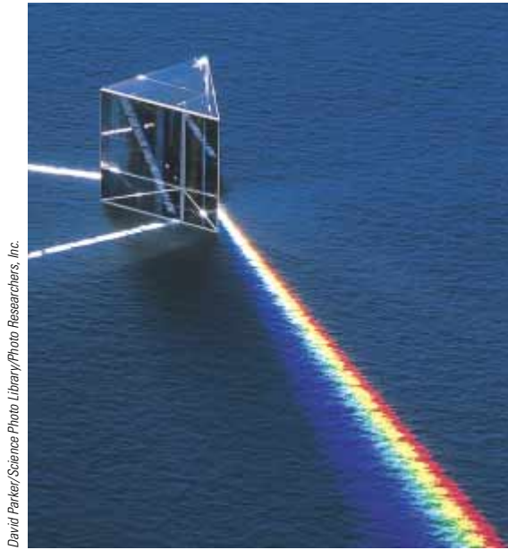
Figure 35.22 White light enters a glass prism at the upper left. A reflected beam of light comes out of the prism just below the incoming beam. The beam moving toward the lower right shows distinct colors. Different colors are refracted at different angles because the index of refraction of the glass depends on wavelength. Violet light deviates the most; red light deviates the least.
