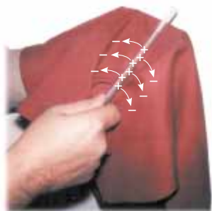
Figure 23.2 When a glass rod is rubbed with silk, electrons are transferred from the glass to the silk. Because of conservation of charge, each electron adds negative charge to the silk, and an equal positive charge is left behind on the rod. Also, because the charges are transferred in discrete bundles, the charges on the two objects are \pm e , or \pm 2e , or \pm 3e , and so on.
