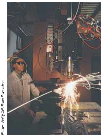
Figure P34.23 A laser cutting device mounted on a robot arm is being used to cut through a metallic plate.
