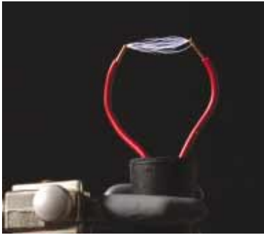
Figure 26.16 Dielectric breakdown in air. Sparks are produced when the high voltage between the wires causes the electric field to exceed the dielectric strength of air.
