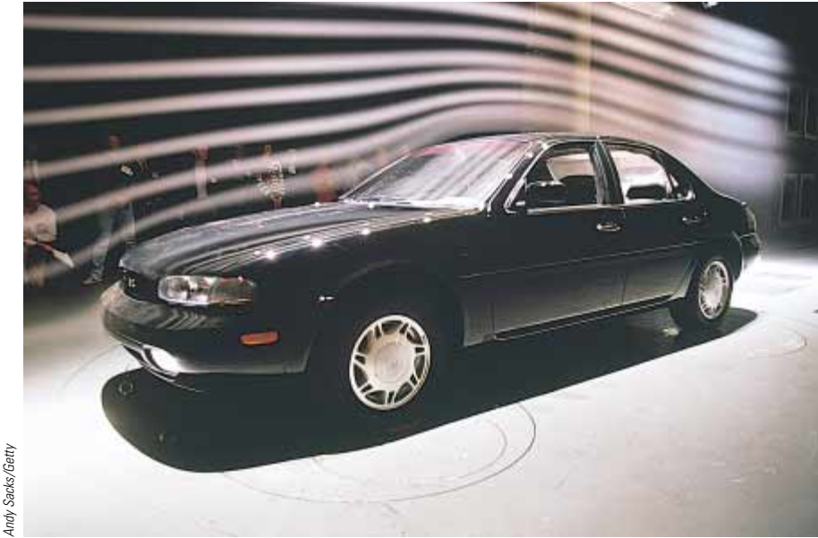
Figure 14.14 Laminar flow around an automobile in a test wind tunnel.
