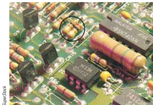
Figure 27.6 The colored bands on a resistor represent a code for determining resistance. The first two colors give the first two digits in the resistance value. The third color represents the power of ten for the multiplier of the resistance value. The last color is the tolerance of the resistance value. As an example, the four colors on the circled resistors are red (= 2), black (= 0), orange (= 10^3 ), and gold (= 5%), and so the resistance value is 20 \times 10^3 \Omega = 20 \text{ k}\Omega with a tolerance value of 5% = 1 k \Omega . (The values for the colors are from Table 27.2.)
