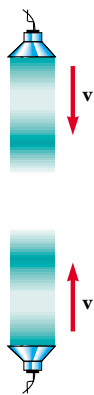
Figure 18.7 Two speakers emit sound waves toward each other. When they overlap, identical waves traveling in opposite directions will combine to form standing waves.
