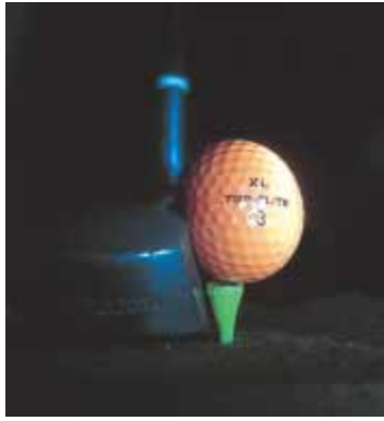
Figure 9.5 (Example 9.3) A golf ball being struck by a club. Note the deformation of the ball due to the large force from the club.
