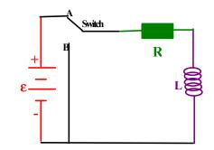
where I(t) is a function of time. If the switch is closed (position A) at t=0 and I(0)=0 (assuming the current is zero at t=0) then
