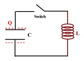
At t = 0 the switch is closed and a capacitor with initial charge  $Q_0$  is connected in series across a inductor (assume there is no resistance). The initial conditions are  $Q(0) = Q_0$  and I(0)= 0. Moving around the circuit in the direction of the current flow yields
