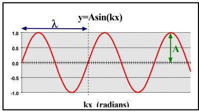
$y = Asin(k(x-vt) = Asin(kx-\omega t))$  where  $\omega = kv$  ( $v = \omega/k$ ). The period of the oscillation,  $T = 2\pi/\omega = 1/f$ , where f is the linear frequency (measured in Hertz where 1Hz = 1/sec) and  $\omega$  is the angular frequency ( $\omega = 2\pi f$ ). The speed of propagation is given by  $v = \omega/k = \lambda f$ .
