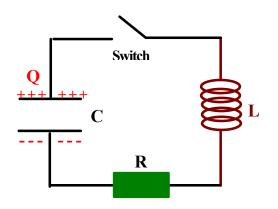
At  $\mathbf{t} = \mathbf{0}$  the switch is closed and a capacitor with initial charge  $\mathbf{Q}_{\mathbf{0}}$  is connected in series across an inductor and a resistor. The initial conditions are  $\mathbf{Q}(\mathbf{0}) = \mathbf{Q}_{\mathbf{0}}$  and  $\mathbf{I}(\mathbf{0}) = \mathbf{0}$ . Moving around the circuit in the direction of the current flow yields
