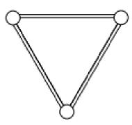
Trusses are typically made of steel, wood, or occasionally a combination of steel and wood. Concrete is seldom utilized for trusses due to its weight. Whether to use steel or wood depends on the type of structure required, the intended aesthetic, and compatibility with the roof framing and roofing materials.
