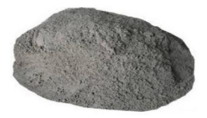
• Slag cement: is a type of cement that contains ground granulated blast furnace slag, which is a byproduct of the iron and steel industry. Slag cement is more resistant to sulfate attack and has a lower heat of hydration than Portland cement.
