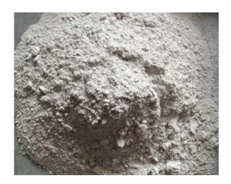
• White cement: is a type of cement that is made from white-colored raw materials. White cement is used for decorative purposes, such as in white concrete and terrazzo.
