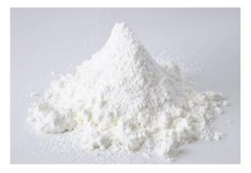
• Expanding cement: is a type of cement that expands when it hardens. Expanding cement is used in applications where it is important to minimize shrinkage, such as in precast concrete and repair mortars.
