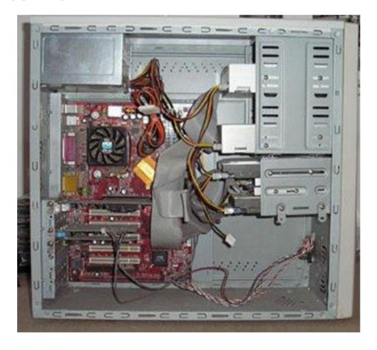
**Motherboard:** It is an electronic board to which all components of the computer are connected, meaning its role the basic thing is to connect computer components together, organize their work, and transfer data among them.
